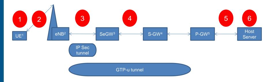
1: User Equipment - 2: evolved NodeB (LTE radio base-station) - 3: IP Security gateway - 4: Serving Gateway - 5: Packet data-network Gateway
